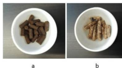
Figure 2: Representation of raw materials used in gasification: (a) pellets of coffee grounds; (b) pellets of lignocellulosic biomass.
