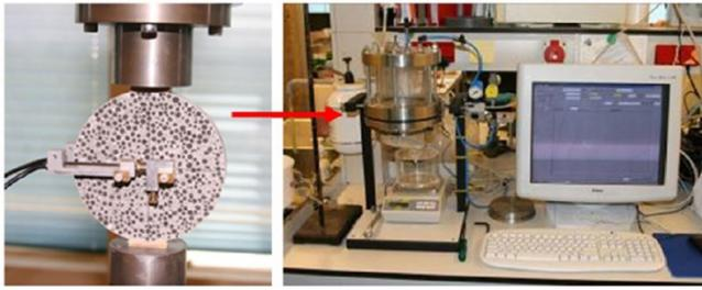
Pre-cracking of the concrete slab and subsequent permeability testing 0.
