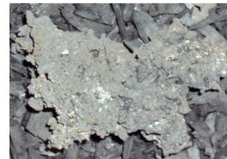
Fig. 2. Stones formed in the reactor after gasification of mixtures containing SS.
