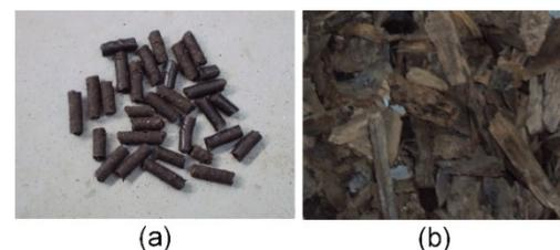
Wastes for gasification tests: (a) pelletized SS and (b) WW chips.
