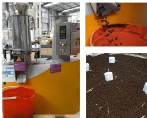
Figure 1: Representation of the process of pelleting; the pelletizer is represented in the image on the left, and the pellets in the two images on the right.
