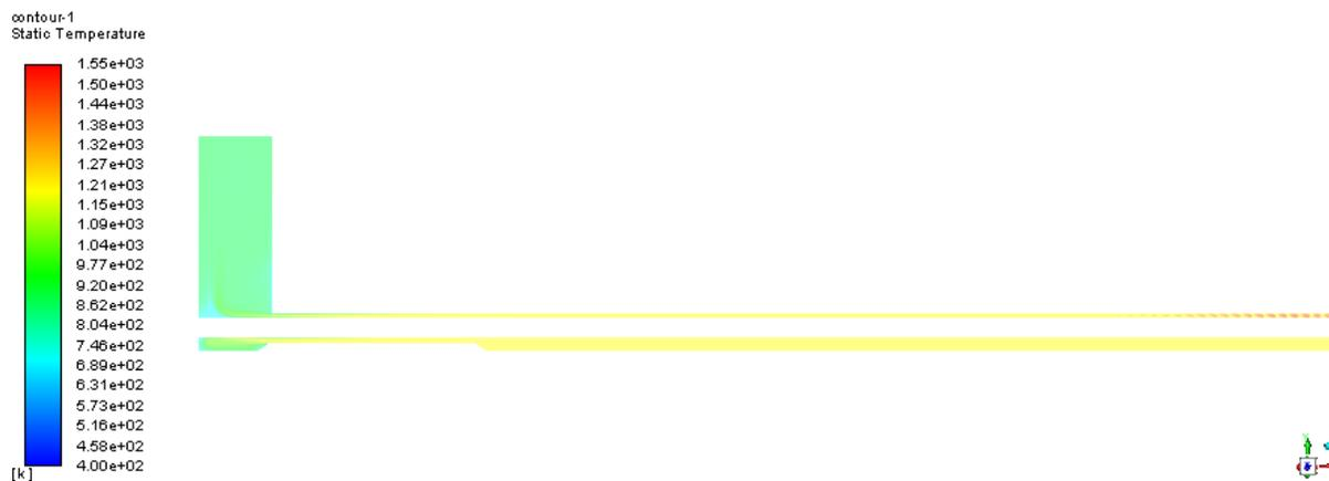
Temperature field along a longitudinal section of the furnace
