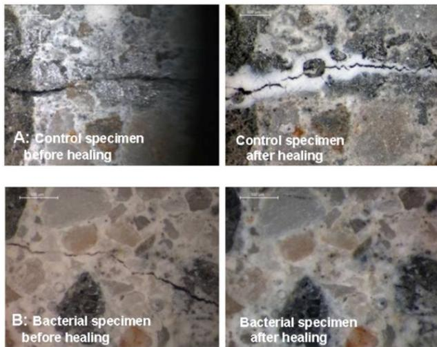
Images of pre-cracked control (A) and bacterial (B) concrete specimen before and after healing [6].
