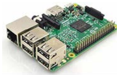
Figura 3 La Raspberry Pi 3 B+.
