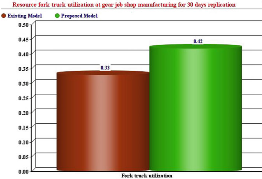
Fig. 11.29 Comparison between resource fork truck utilization among existing and proposed model for 30 days replication
