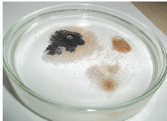
Figure 14. Behavior on water surface: usual sand, sand with a polyurethane film and hydrophobic sand
