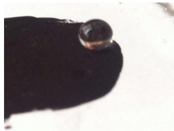
Figure 12. Behavior of water drop on a glass surface with layer of the applied hydrophobic soot.
