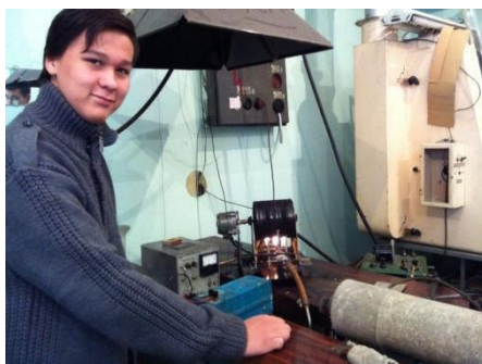
Figure 10. Installation for receiving superhydrophobic soot
