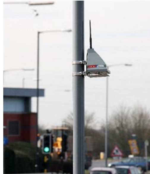
Figure 2: Outdoor AQmesh unit
