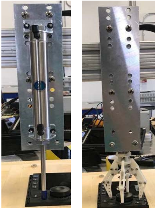
Figure 4. a) Key press test structure. b) Gripper rotary structure
