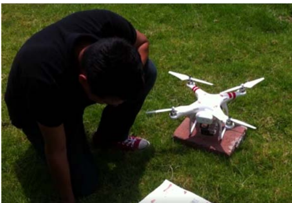
Figure 2 Drone used with NIR camera.
