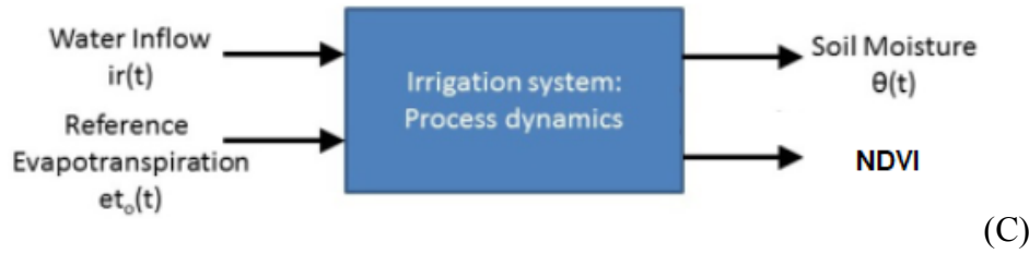
Fig. 4: Irrigation system input/output definition: (A) [7] proposed system, (B) system addition, and (C) final model.
