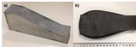
Figure 2. Wedges a) As machined & b) After forging.
