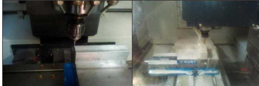
Image 7. CNC machining of wing support.
