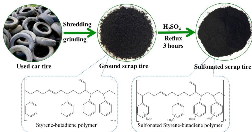
Scheme 1. Preparation of sulfonated waste tire rubber (WTR-SO 3 H) and the possible structure of the pristine styrene-butadiene polymer and the sulfonated styrene-butadiene polymer.
