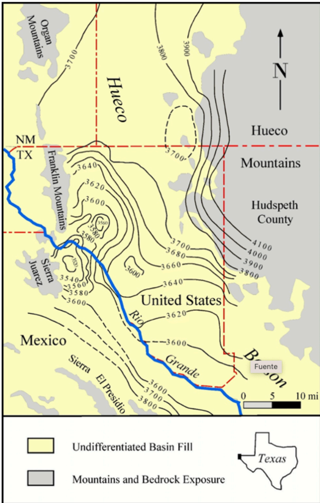
FIGURE 2: Hydraulic head map showing groundwater movement down the axis of the Hueco Bolson to discharge areas near the Rio Grande. Drawdown cones of depression have been formed by over-pumping by the City of El Paso and Ciudad Juarez, and an artificial groundwater divide is formed between the two cities north of the International boundary (3580 ft contours) (modified from Hibbs et al., 1997 and Hibbs, 1999).
