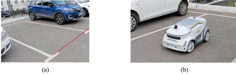
Figure 5. (a) Parking slot in a real parking area (the marking line is highlighted with a red dotted line), (b) the parked Avrora Unior robot.
