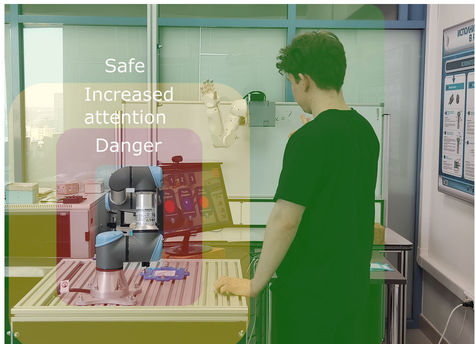
Fig. 4 The hazard zones layout diagram: Danger zone (red), Increased attention zone (yellow), Safe zone (green)
