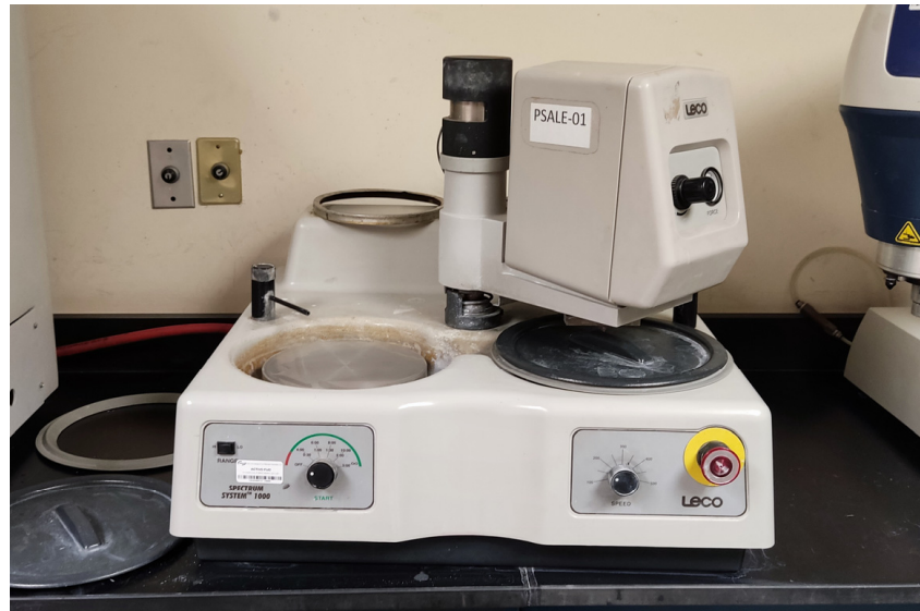
Figure 2. Device used to sand pieces.
