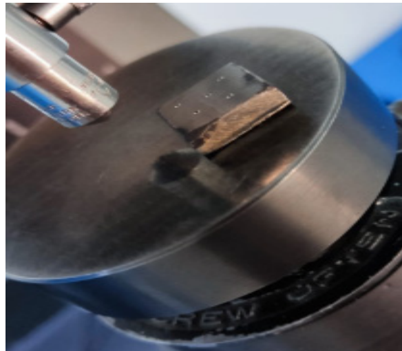
Figure 6. Hardness test points applied to the specimen.
