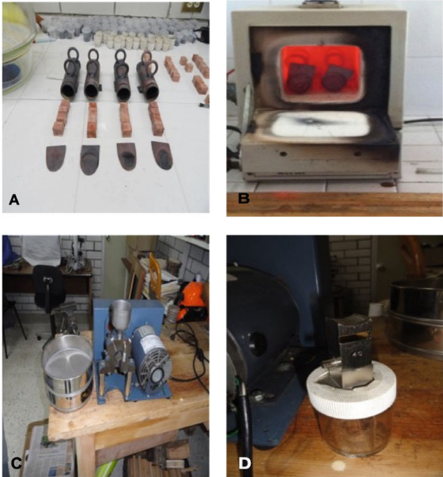
Fig. 3 (a) Placement of the firewood samples in the iron tubes, (b) Elaboration of the charcoal in the muffle at 750 °C, (c) Grinding of charcoal and (d) Screening of charcoal
