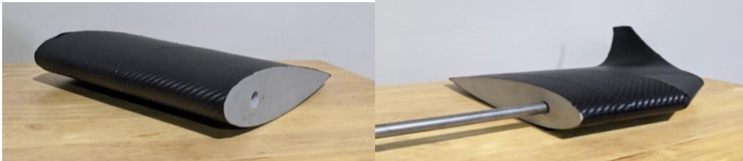
Figure 15: Final wing assembly without winglet
