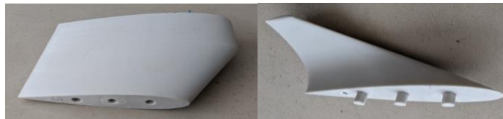
Figure 12: Part 2 of wing with winglet.
