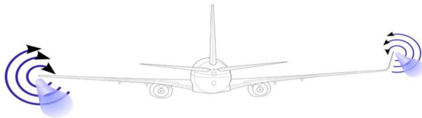
Figure 6: Effect of winglets on vortex formation [21].
