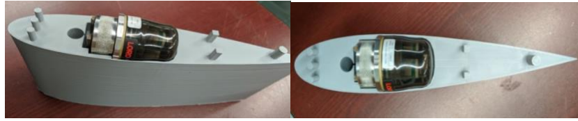
Figure 14: Sensor assembly in half wing
