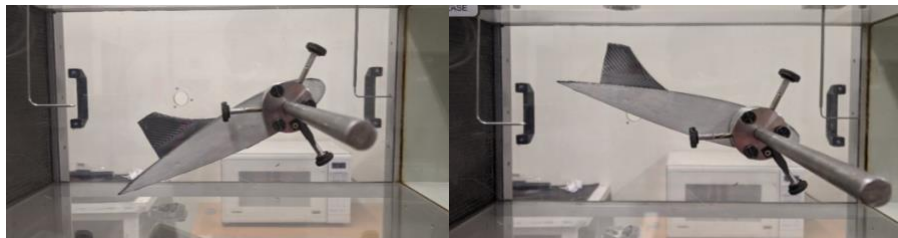
Figure 26: Wing with winglet at 25-degree AOA. Figure 27: Wing with winglet at -15-degree AOA.
