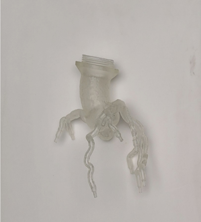
Fig. 1. Aortic artery adapted for integration into the hydraulic system.
