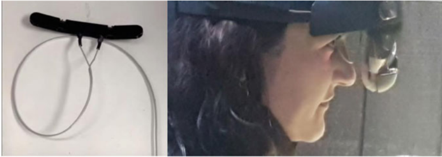
Fig. 11.4 The SMA actuator set into the HoloLens 2 visor
