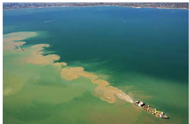
Fig. 1 Turbidity of seawater due to the diffusion of dredged materials (short-term impact) (Saremi 2014)
