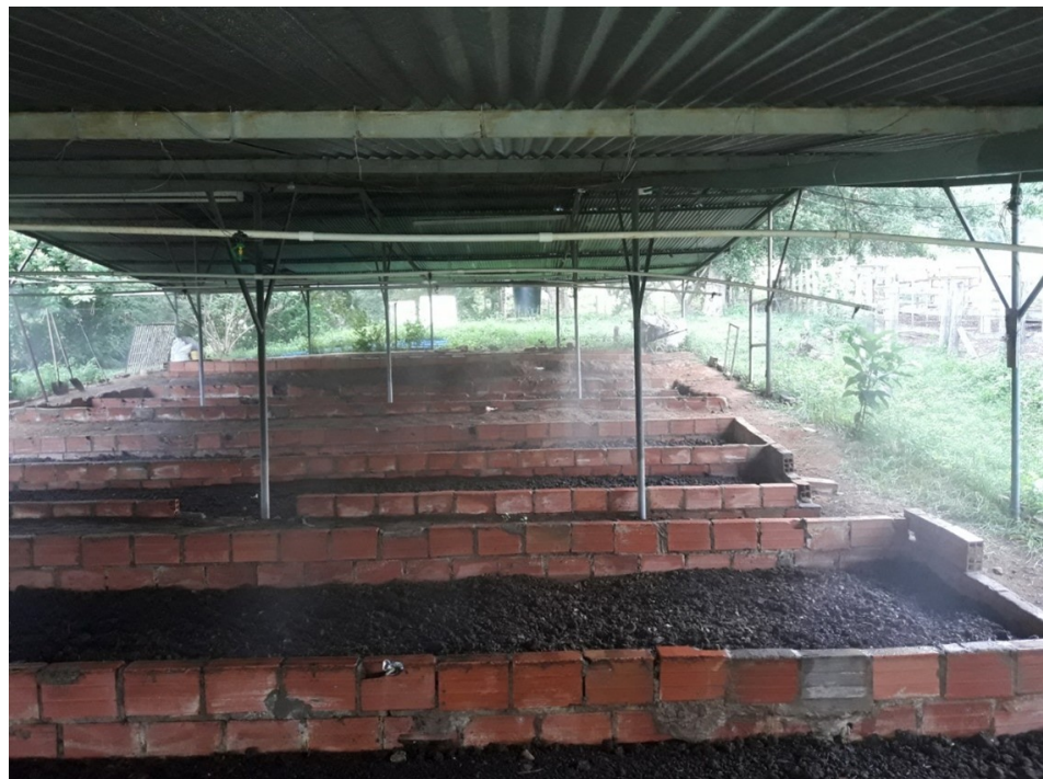
Figure 6. Test of the automated irrigation system for the control of the humidity and temperature variables.
