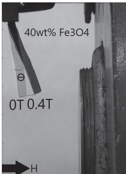
Fig. 1 Deflection of 40wt% magnetite-PVA Ferrogel under an increasing magnetic field(H)
