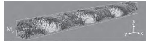
Figure 1—The double helix configuration at the zero-field state of the magnetization reversal of a 150 nm diameter NiFe wire.
