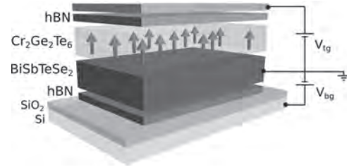
Fig.1. Schematic of the device geometry and electrostatic gating geometry. TI and 2D magnet flakes with few-layer thickness are double-encapsulated between hBN layers on a Si/SiO 2 substrate.
