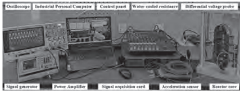
Fig.1. Vibration testing platform for anodic saturable reactor core
