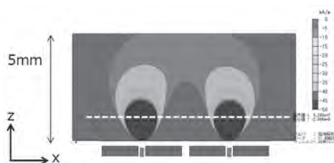
Fig.2 SDF of the sensor with 2-mm MFC. Broken line indicates the sample-sensor distance of 1 mm.
