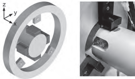
Fig. 2. Schematics for application of spin Hall magnetic field sensor to a rotor.
