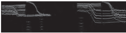
Fig. 1. Spin-orbit-torque-induced multi-level states. The current-induced magnetization switching hysteresis shows systematic dependence on the magnitude (a) and deviation angle from the film plane (b) of the bias field.
