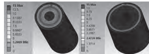
Fig 2. Results of mechanical stiffness analysis of the Conventional model (left) and slotless model (right)
