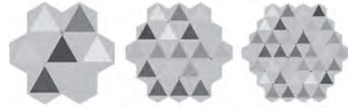
Fig 1. Illustration of the model. The green regions are of low damping allowing for the spin wave propagation. The colored triangular regions have higher damping to absorb spin wave. STNOs are shown as the small dots.
