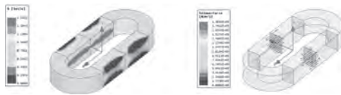
Fig.2. The distribution of magnetic induction intensity and volume force density vector in the core of anodic saturable reactor.
