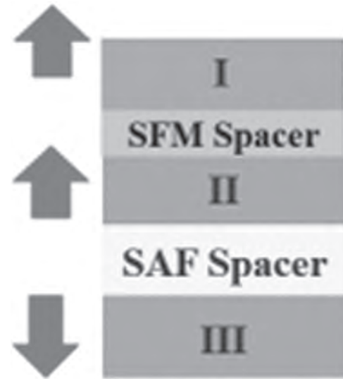
Fig.1 HFL design with top MTJ.
