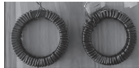
Fig.2 Magnetic properties test samples of amorphous alloys
