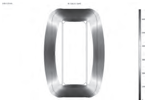
Fig. 2. Medium-high frequency transformer core deformation of ultra-thin oriented silicon steel (GT-100) caused by magnetostrictive force ( B = 1.2T , f = 1kHz )
