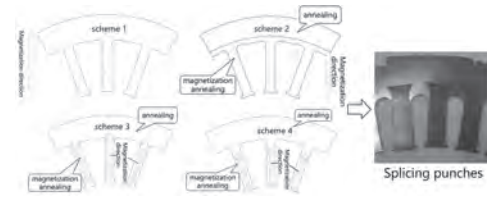
Fig.1 Four splicing schemes and stator punching
