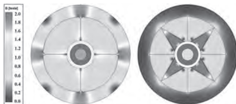
Fig. 1. Magnetic flux density distribution of conventional model and proposed model
