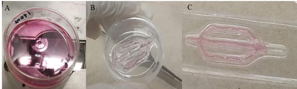
Figure 5 Cell seeding results, (a) culture dishes seeding (b) PDMS channels in 35 mm culture dishes model seeding (c) PDMS OoC on slides model seeding (see online version for colours)
