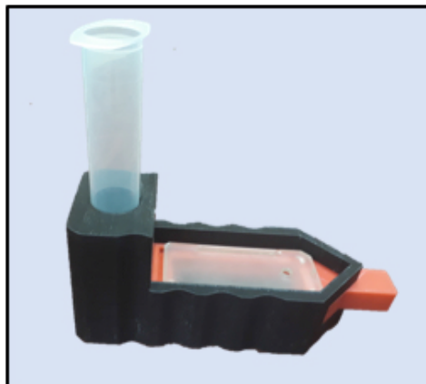
Figure 7 Final assembly of the OOC system (protective vessel and irrigation system) (see online version for colours)
