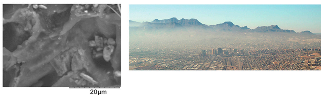
Figure 1. (Left) Scanning electron microscopy image of particulate aerosols, which are among the most common on the region, particle size can range from nanometers to microns. (Right) Panoramic photograph on a high-polluted day at El Paso-Juárez region, one can observe a clear dusty cloud suspended at the atmosphere (Image credit: https://www.quora.com/ [What is the air pollution like in El Paso, TX?] ).
