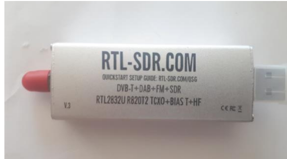
Figure 6. RTL-SDR to analyze the hydrogen line.
