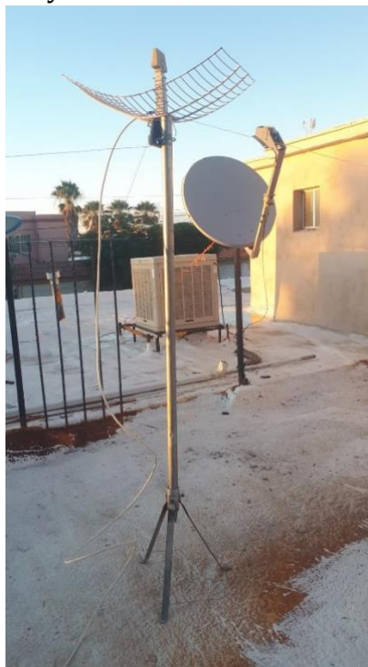
Figure 2. Parabolic grid antenna at front and cable antenna at back.
