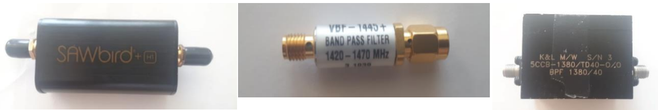
Figure 5. LNA at left, 1445 MHz BPF at middle, and 1380 MHz BPF at right.
