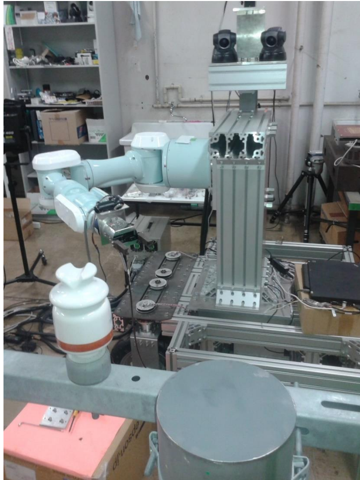
Fig. 1. Prototype in Tatsuno Laboratory illustrates the UP, manipulator robot and stereo vision system.
