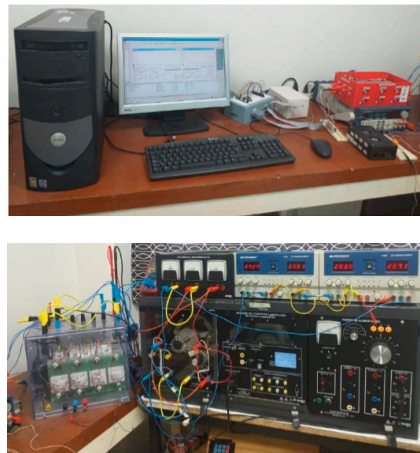
Figure 8. Hardware for the DC motor velocity controller.
