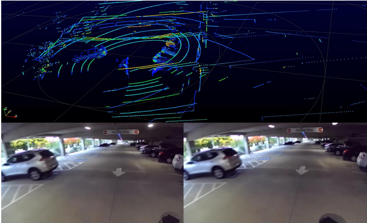
Figure 51. Images obtained by the rear VLP-16 sensor and rear ZED camera, inside a parking lot – section B.
