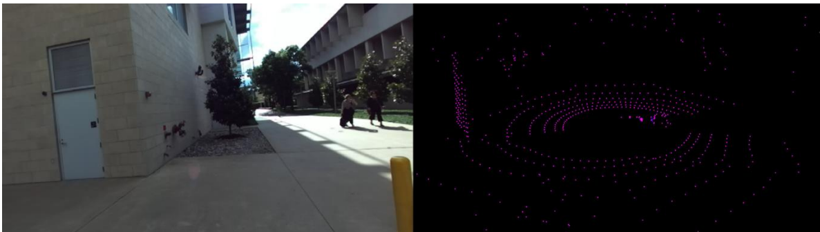
Figure 39. Erroneous representation of depth.
