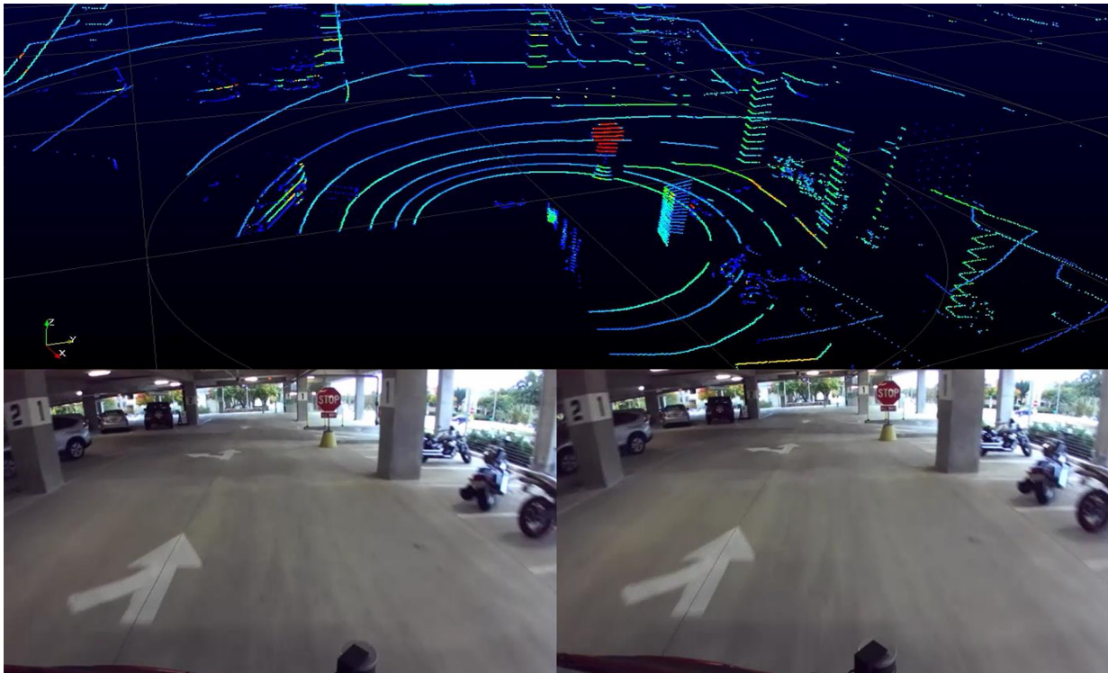
Figure 49. Images obtained by the front VLP-16 sensor and front ZED camera, inside a parking lot – section B.
