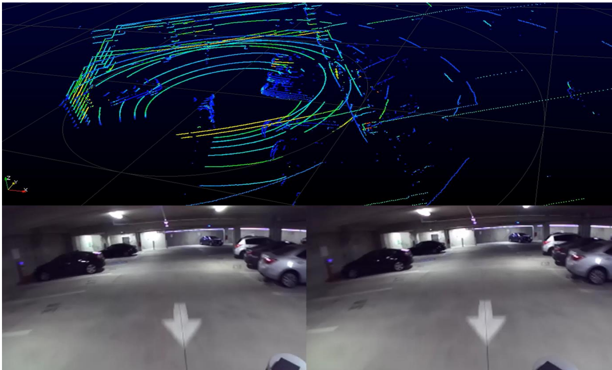
Figure 51. Images obtained by the rear VLP-16 sensor and rear ZED camera, inside a parking lot – section B.
