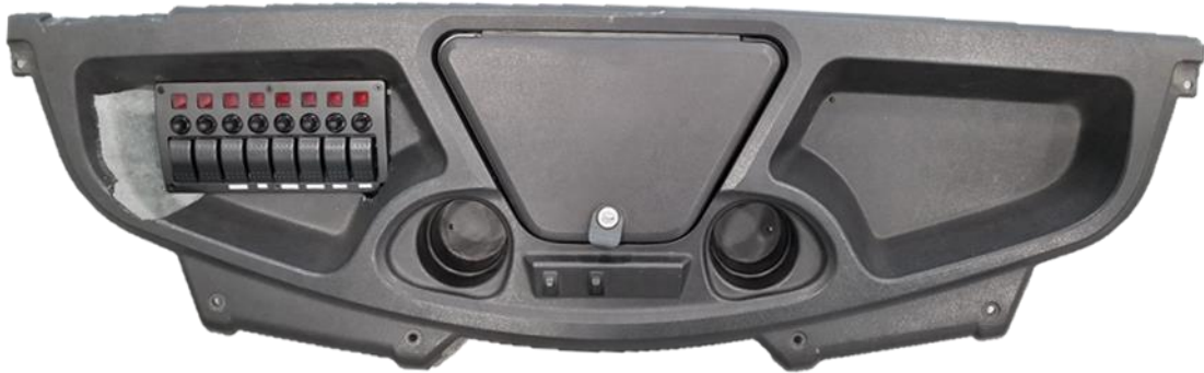
Figure 17. Electrical switch installation.
