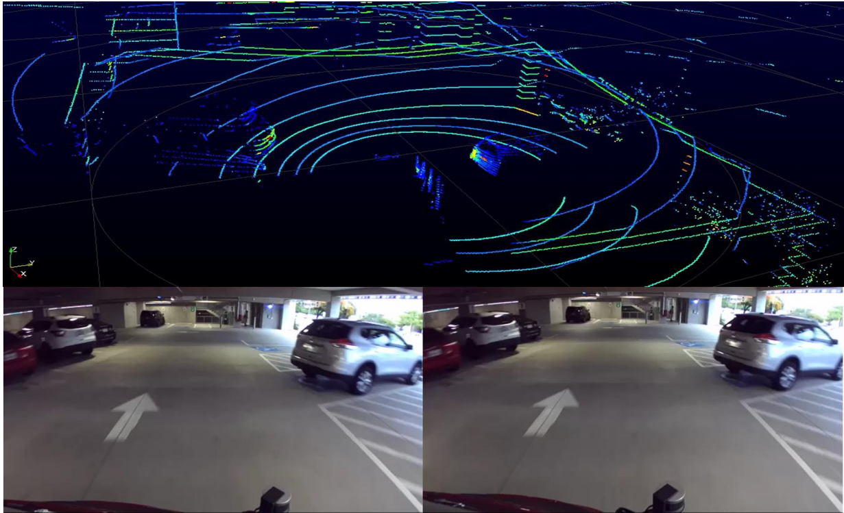
Figure 49. Images obtained by the front VLP-16 sensor and front ZED camera, inside a parking lot – section B.
