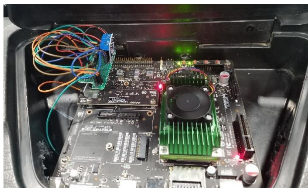
Figure 21. Jetson TX2 Installation.
